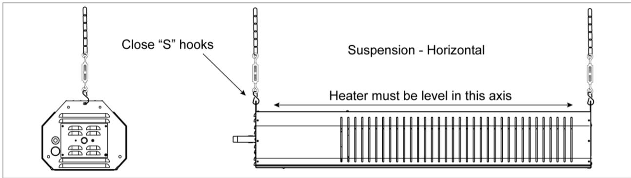
Diagram below shows the possible chain methods to hang at different angles.
