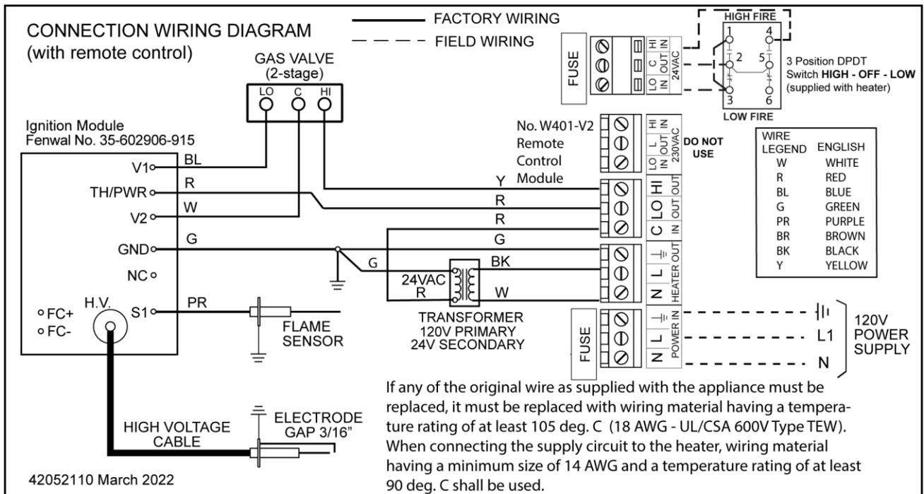
**16.6) FIELD CONNECTION AND WIRING DIAGRAM – 2 STAGE 24V MODELS N3/L3 WITH REMOTE**
