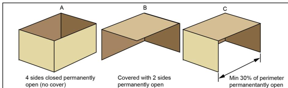
**⚠ WARNING** For the purposes of clearances to combustibles and ventilation all applications not classified as outdoors according to the definitions above shall comply with the requirements for indoor installations.
