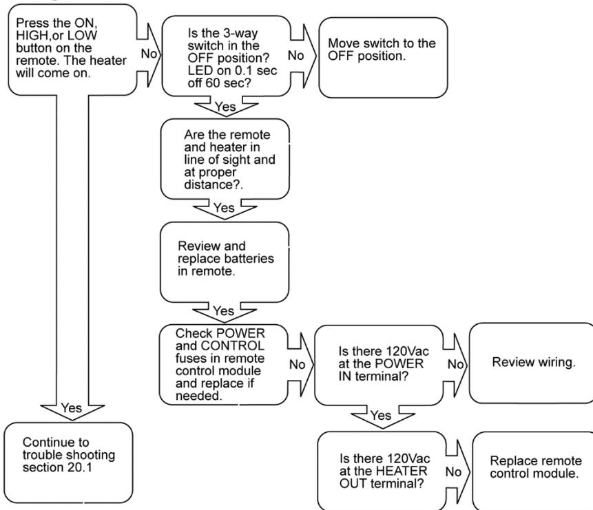
Using 3-way position switch:
