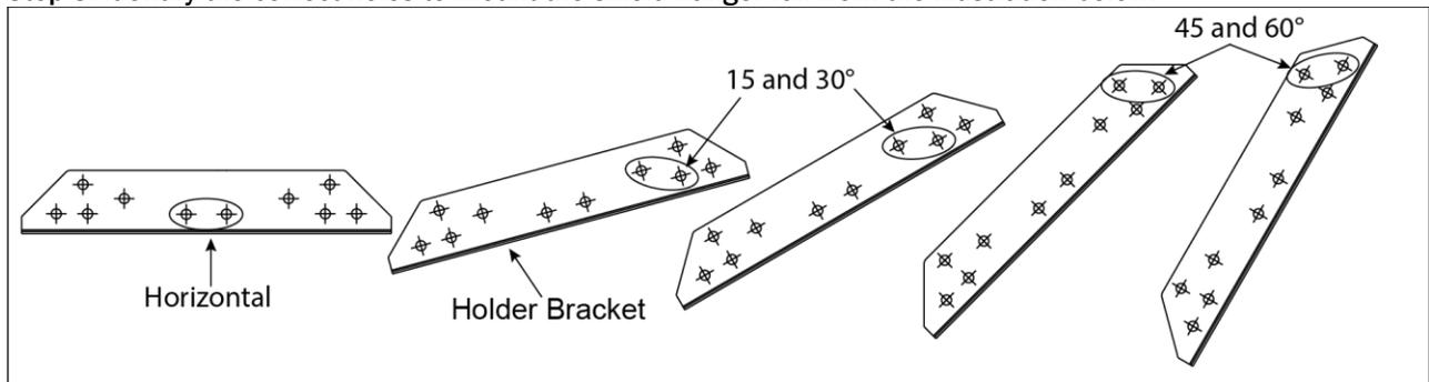
Step 4. Attach the heat shield hanger rail to the holder bracket using (2) black oxide #8 screws on each end. Horizontal position shown below.
