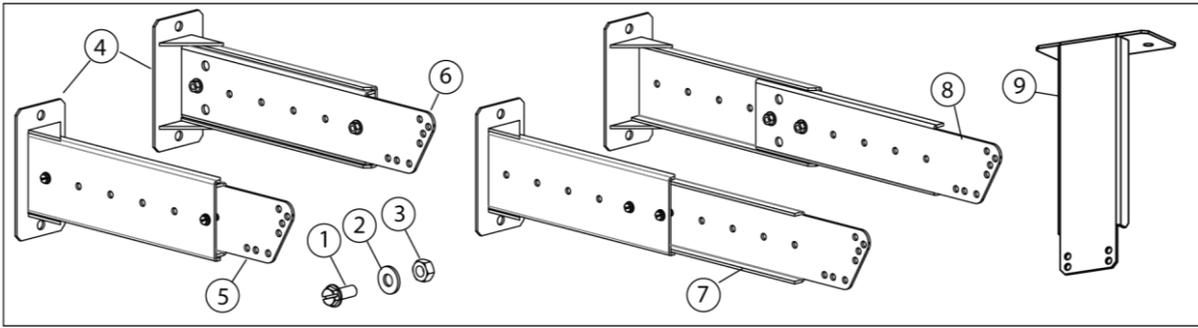
The tables below can be used to select the correct bracket to ensure that the heater is installed at the correct clearance to combustibles distance from the ceiling depending on whether the heater is installed indoors or outdoors, the mounting angle and whether a heat shield is installed.
