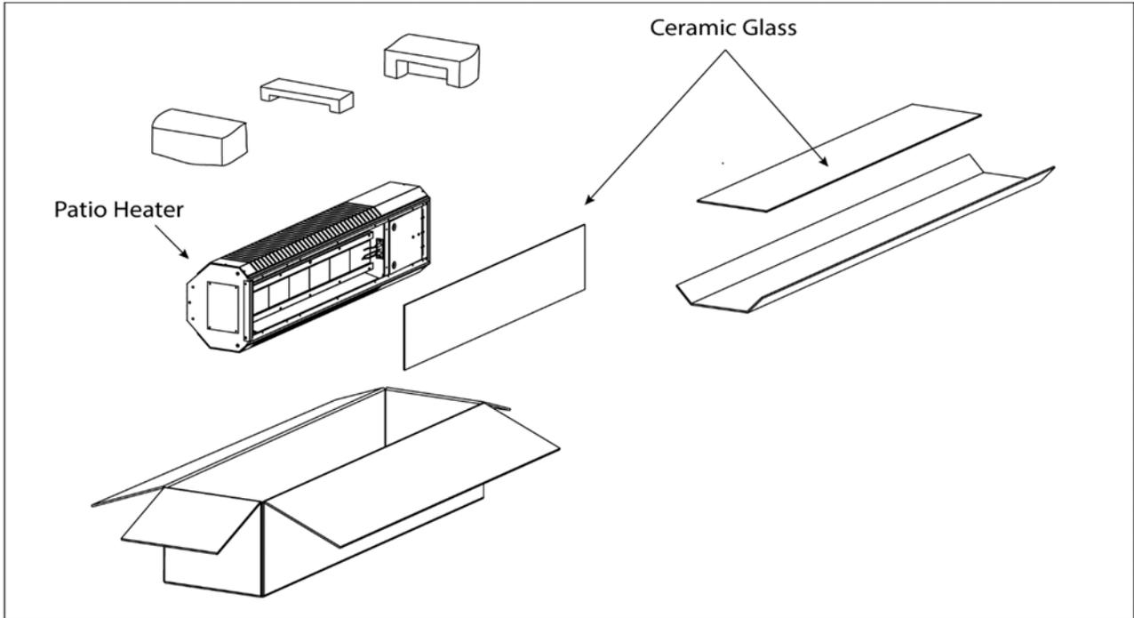
**⚠ CAUTION** It is recommended that two people lift the heater out of the carton. Do not remove from the remaining packaging until the heater is ready to be hung.
