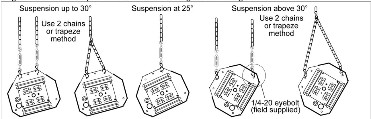
Notes: When suspending at 25 degrees if the heat shield is installed use the 30-degree location for the heat shield.
