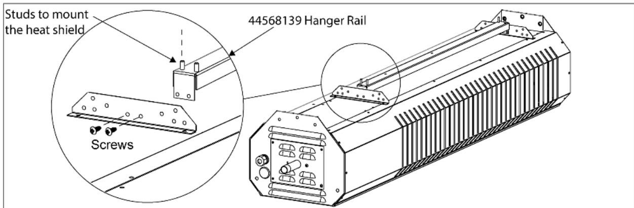
**CAUTION** IMPORTANT: Use the **Acorn nuts** at the control end of the heater as shown in the illustrations so that the heat shield can expand when the heater is turned on. Failure to do so may result in the heat shield distorting.
