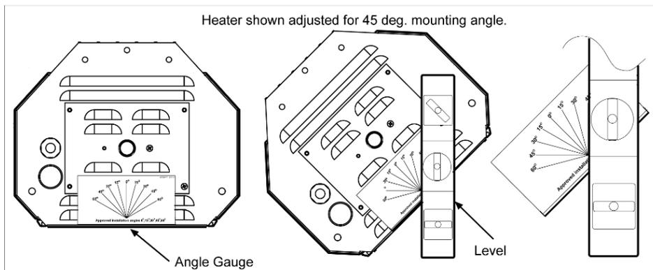
Step 2. Attach the (2) holder brackets to the top of the heater using (2) black oxide #8 screws per bracket.
