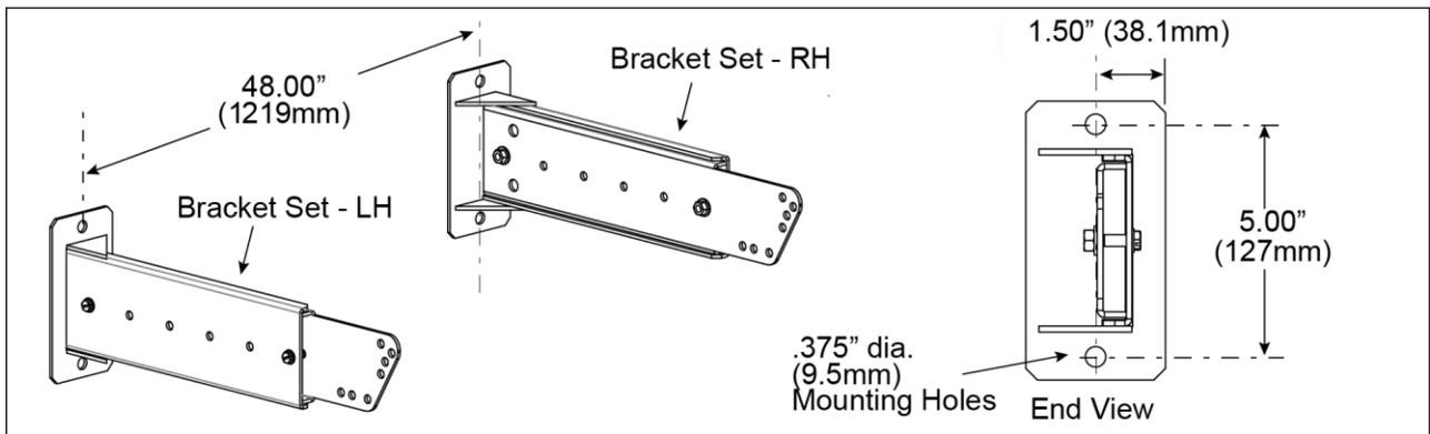
A left-hand LH and right-hand RH bracket must be assembled. Torque screws and locknuts to 5 lb/ft.
