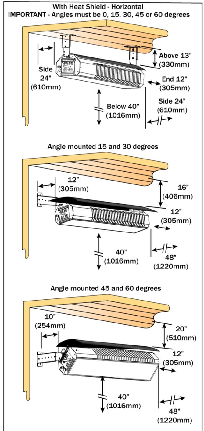
**⚠ WARNING** The stated clearance to combustibles represents a surface temperature of 90° F (50° C) above room temperature. Building materials with a low heat tolerance (such as plastics, vinyl siding, canvas, tri-ply, etc.) may be subject to degradation at lower temperatures. It is the installer's responsibility to assure that adjacent materials are protected from degradation.
