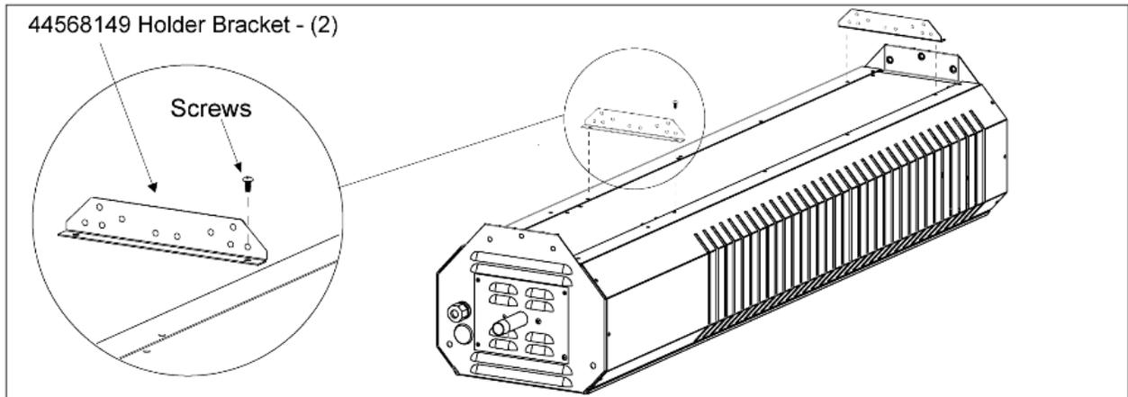
Step 3. Identify the correct holes to mount the shield hanger rail from the illustration below.
