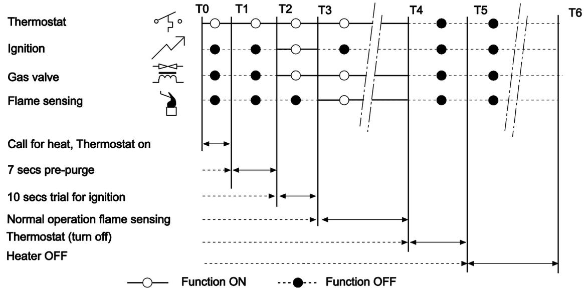
If the burner fails to light, or flame is not detected during the first trial for ignition (a period of 10 seconds) the gas valve is de-energized and the control goes through an inter-purge delay of 15 seconds before another ignition attempt. The control will attempt two additional ignition trials before going into lockout.
