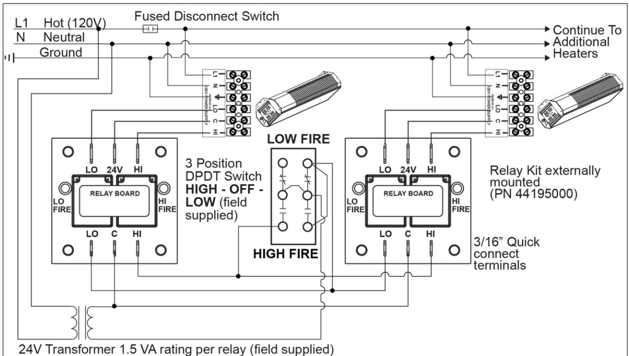
**C. LOW VOLTAGE (24V) THERMOSTAT CONNECTIONS - SINGLE HEATERS**
