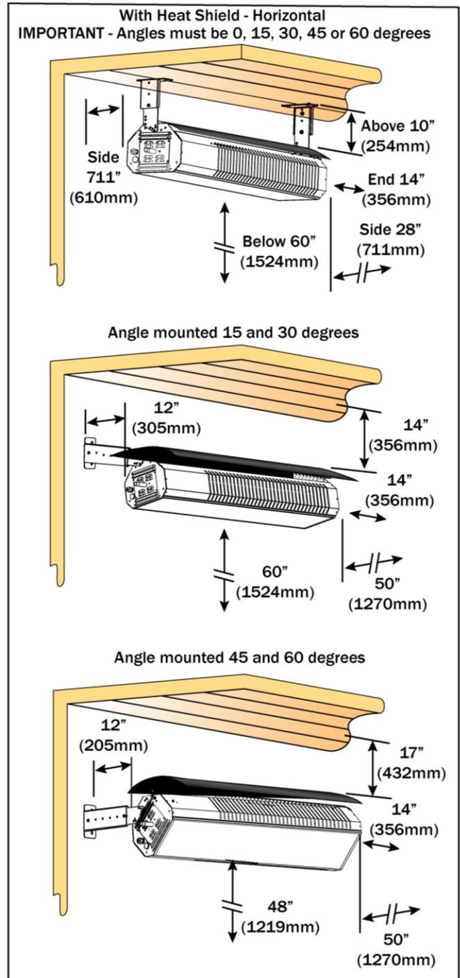
**⚠ WARNING** The stated clearance to combustibles represents a surface temperature of 117° F (65° C) above room temperature. Building materials with a low heat tolerance (such as plastics, vinyl siding, canvas, tri-ply, etc.) may be subject to degradation at lower temperatures. It is the installer's responsibility to assure that adjacent materials are protected from degradation.
