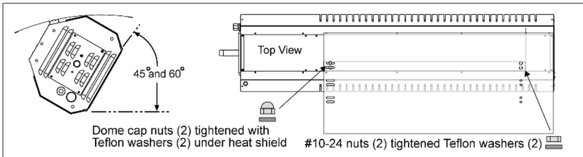
**Note: When in operation the heat shield will deform slightly when installed at a mounting angle of 45 or 60 degrees. This is normal. After operation the heat shield should return to its normal shape.**
